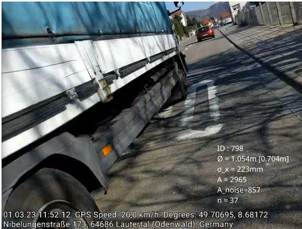
Figure 4.1: shows the screenshot displaying a typical encounter. Notably is that the correlation to Table 4.1 is perfect. The red car was measured, then a timeout occurred, and then the truck was measured. Furthermore it is an interesting example because the red car produced a measurement where the first and strongest reflector basically is the same distance, while the truck produced a measurement where the first and strongest reflector are significantly different. This is the reason why we will use the first reflector in the following analysis. Since the measured distance of the first reflector correlated better with the intended use case.
