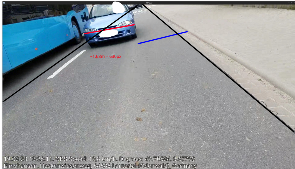
Figure 6.10: oncoming traffic example representing a value measurement. Google Lens identified the car as a Mitsubishi colt of the fifth generation with a width of 1.68m (Without mirrors). A rough estimation let us conclude that in this case the remaining street width is approximately 1.68m as well.
