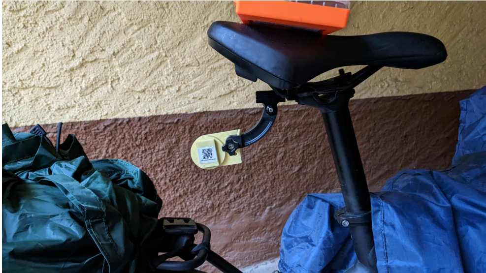
Figure 6.5: Picture of the mounted sensor. The sensor is mounted under the saddle, and the power supply can be either an external powerbank, an integrated 5V battery or any other supply such as compatible e-bikes and phones. The handlebar width to each side is 0.35m, resulting in a total width of 0.7m. This means the sensors measurements, have to be reduced by 0.35m in order to get the actual distance to the object, because the sensor is mounted in the center. This also compensates for the blindspot of 0.3m that we have due to possible direct leakage of the radar signal.
